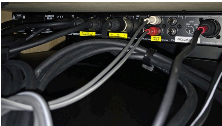
(e) Rear panel labelling allowing quick and simple connection
