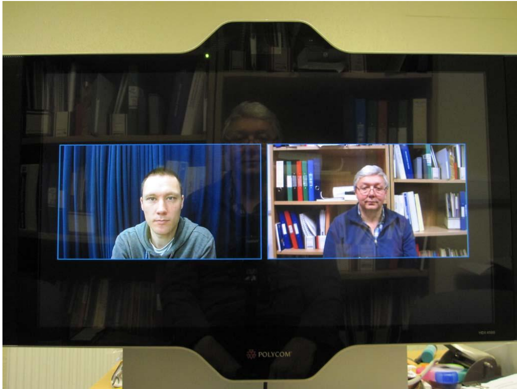
Point to Point Call, Picture outside Picture (POP) no content, near and far sites side by side
