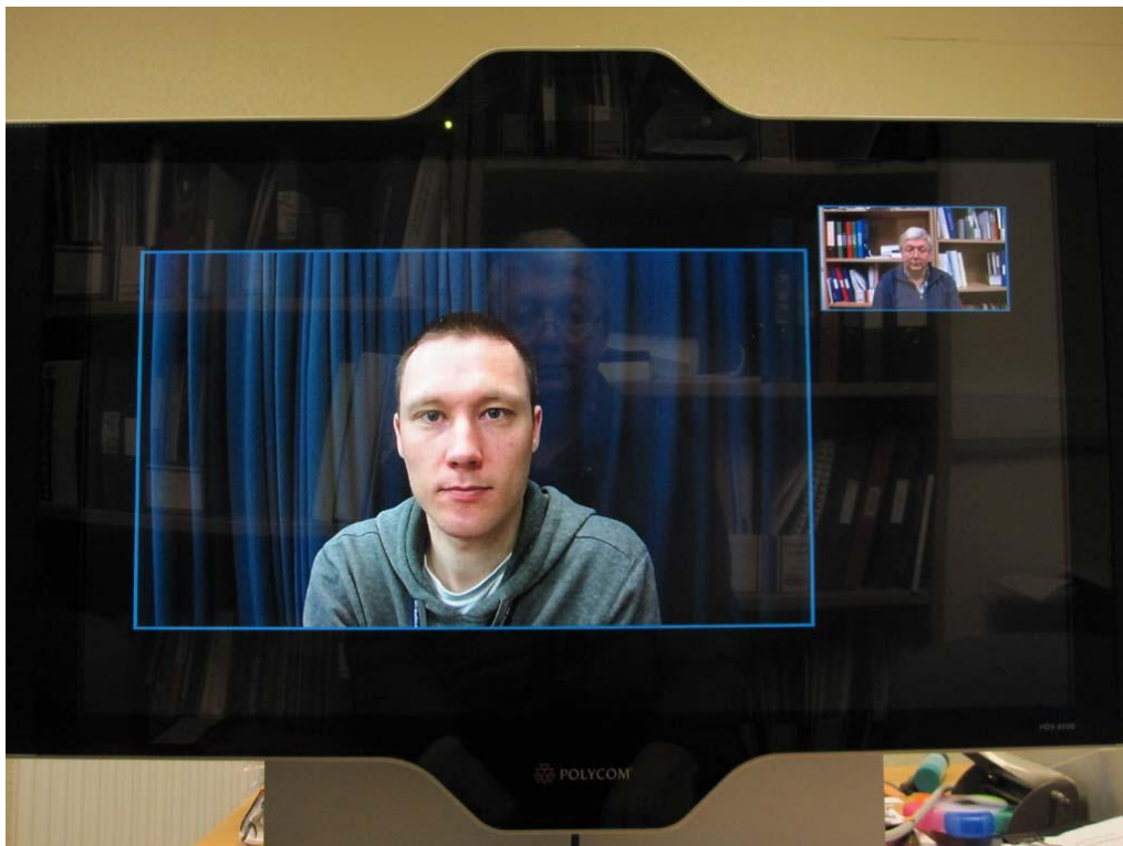
Point to Point Call, Picture outside Picture (POP) no content, far site large, small near site.
