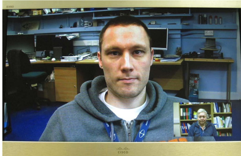
Full screen of the far image with near end Selfview Picture in Picture (PIP)....
