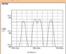
power for each of the three wavelengths within its 50GHz channel The double peaked structure of the central 100Gbit/s wavelength is a feature of the modulation technique used in the prototype equipment. Comparing the two outer peaks, there is also a subtle broadening on the right hand side which is the wavelength carrying the 40Gbit/s signal.
