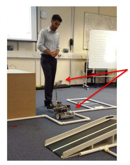
Robot with wireless camera with a TP-Link Nano router to send video streams from robot to remote computer.
