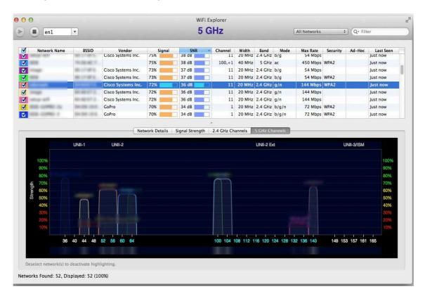
To provide more of a resilient workable solution, improving robustness of the service to help minimise impact of any future interference and eliminating the number of frequent dropouts, it was decided that all future demonstrations should use 5GHz with supported 802.11ac support.
