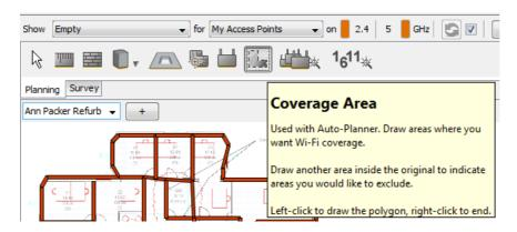
Draw around the walls on the floor plan until the desired area is fully covered, by left clicking on the mouse. Once complete, right click to stop the drawing and you will see a purple dashed border.
