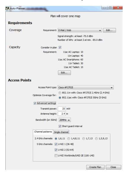
Define your coverage requirements and select the **Capacity** 'Consider in plan' tick box to consider the capacity requirements that were previously configured.
