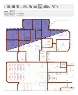
You can also create an exclusion point where no Wi-Fi is required by drawing another coverage area inside the existing one. The exclusion will be marked with a grey box along with a purple dashed border.
