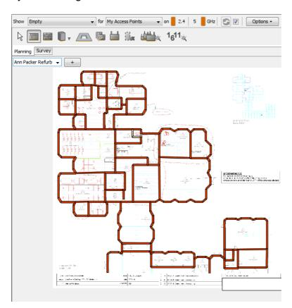
You can fine-tune the floor plans by drawing in doors, windows, furniture etc., by choosing the desired object from the drop down list.
