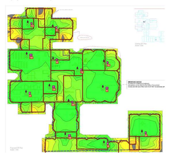
You can tweak by moving the simulated access points by simply selecting and dragging them to a new location on the map.
