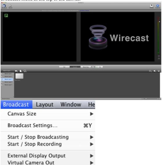
Step 4 Once Broadcast settings has been opened, you can either create a new line for the RTMP server or use the already existing one.
