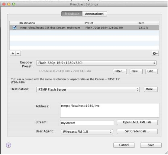
Step 5 Once either a new line or the existing line has been chosen, The destination and other details need to be entered, as can be seen in the image below, I have entered the details given by Streaming wizard to broadcast to the player.
