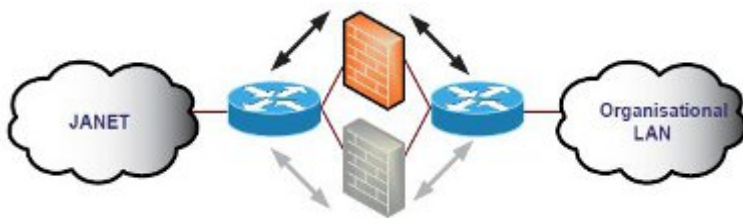
Figure 10: Firewalls in an Active/Passive failover operation
