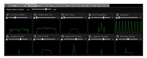
The screenshot below shows the Wi-Fi environment from an open plan office space that has three wireless access points. As the Bluetooth pattern signature is enabled from the Signatures tab above you can see below that there is a strong presence of Bluetooth across all channels 1-13.
