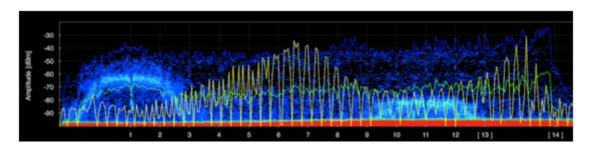
The sweep spectrogram below also illustrates the interference caused by the microwave oven. This lasted for a short period of time - under a minute. The interference can be seen by
