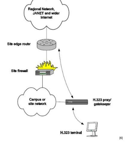
Figure 3: Pass-through topology for a site H.323 proxy/gatekeeper deployment
