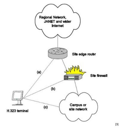
Figure 1: Options for H.323 terminal connection topology
