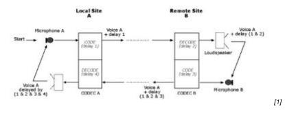
Figure C. 1: Echoes due to CODEC delays
