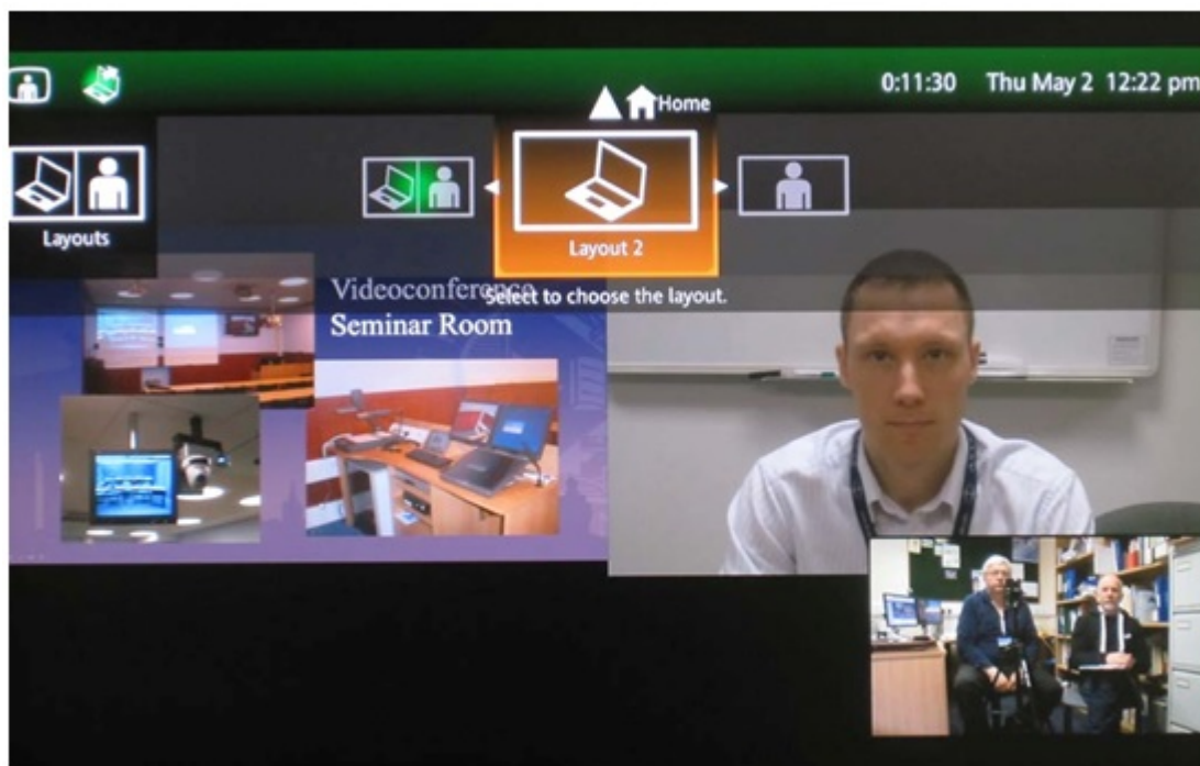
Side by Side Presentation and Far Images, Near Image PIP With Layout Selection Menu
